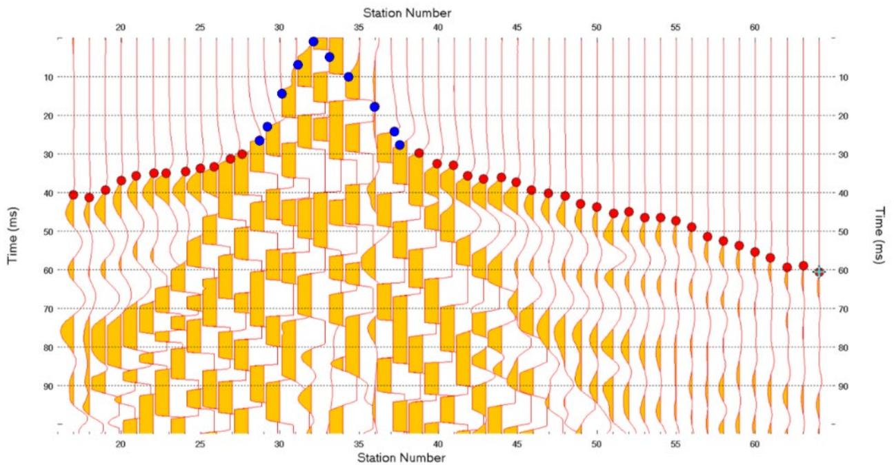
**Fig. S1.** Demonstrative seismogram with first occurrences of seismic waves. Geophone spacing at 2 m, 24 ch apparatus. Blue dots denote occurrences of direct waves. Red dots denote occurrences of refracted waves.
