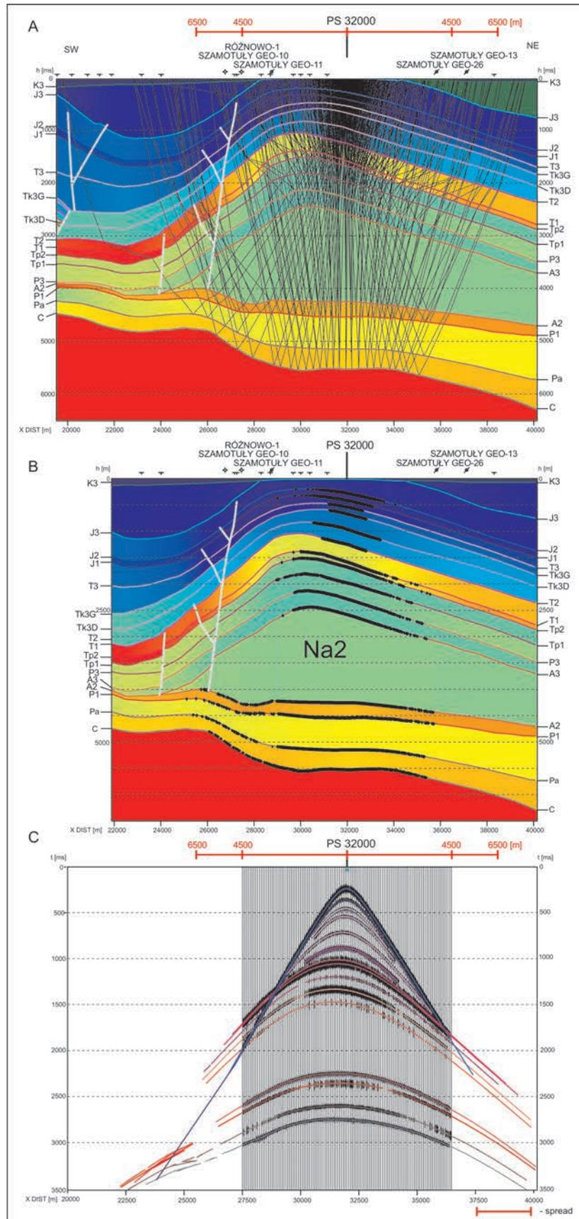
**Fig. 10.** Offset modelling: part of basic, seismic-geological model I (Rogoźno Salt Pillow), PS 32000. **A** – Seismic ray trajectories; **B** – “Lighting” boundaries seismic rays; **C** – Seismic record. Hodographs of reflection waves, marked with colours: Jurassic boundaries – blue; Triassic boundaries – violet; Zechstein boundaries – orange; inside Rotliegend boundary – brown, and bottom of Carboniferous – black
