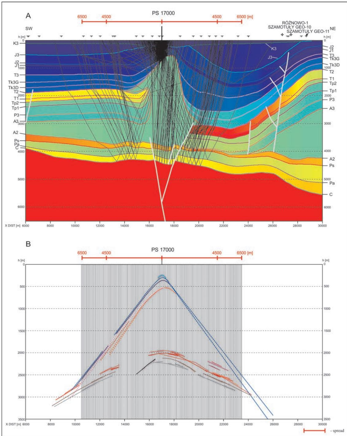
**Fig. 12.** Offset modelling: Szamotuły Salt Diapir model (V), PS 17000. **A** – Seismic ray trajectories; **B** – Seismic record. Colours marked as in Fig. 10C
