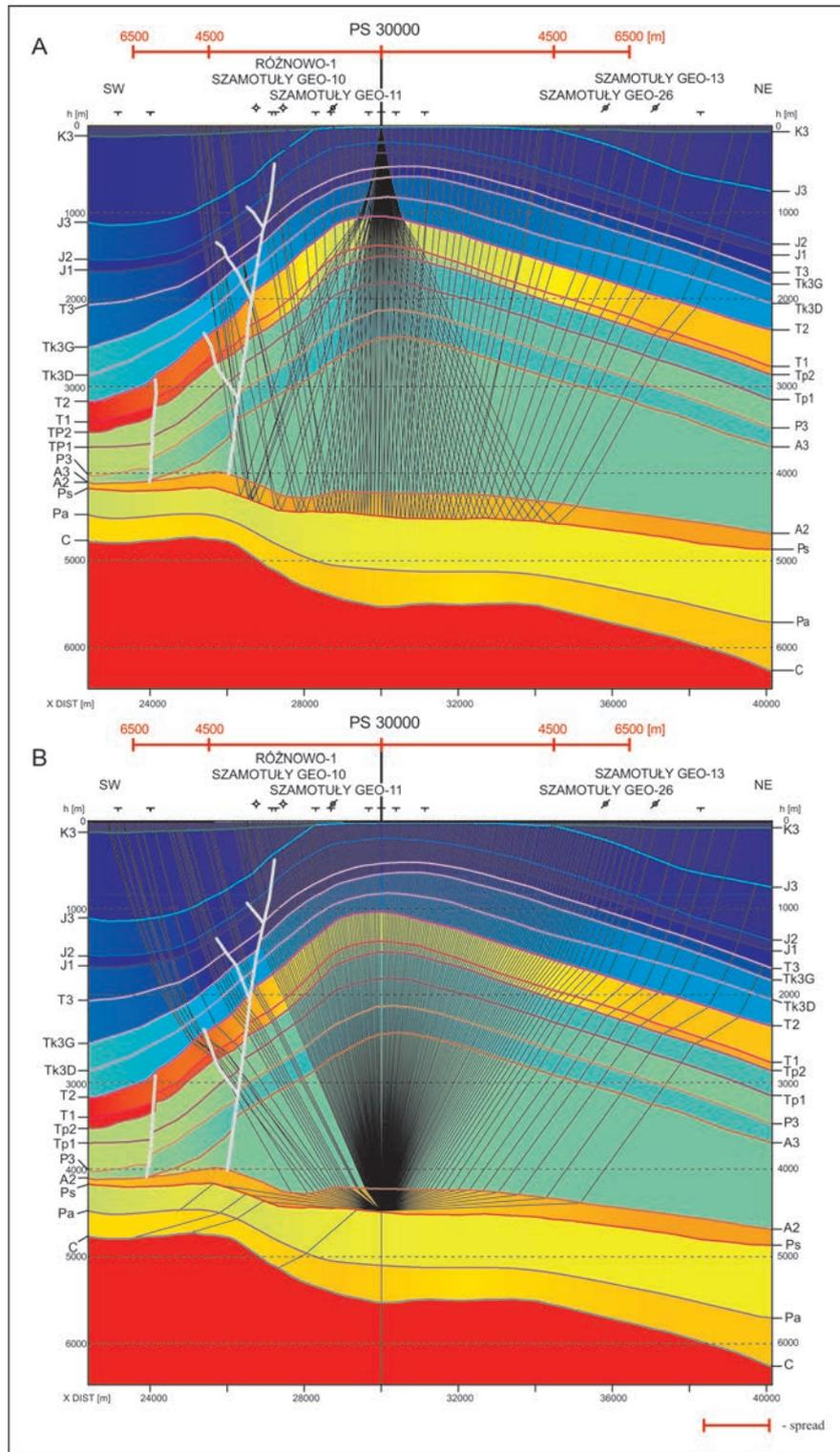
**Fig. 16.** Seismic ray trajectories, Salt Pillow Rogoźno, PS 32000. **A** – shot record simulation; **B** – diffraction point (CDP gather simulation)
