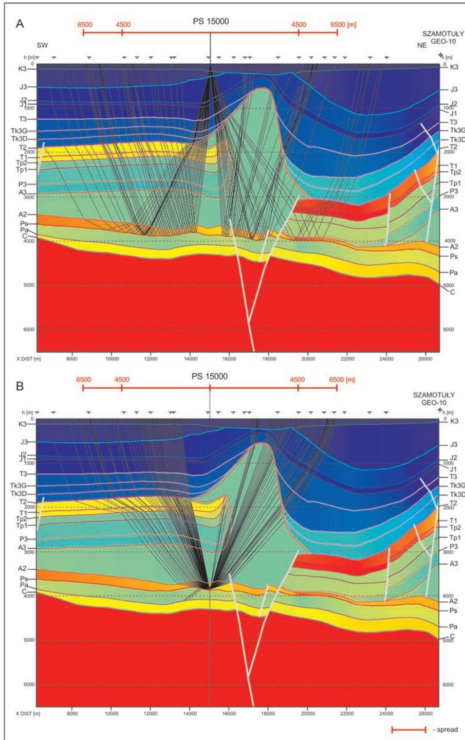
**Fig. 14.** Seismic ray trajectories, Szamotuły Salt Diapir model (V), PS 15000. **A** – shot record simulation **B** – diffraction point (CDP gather simulation)
