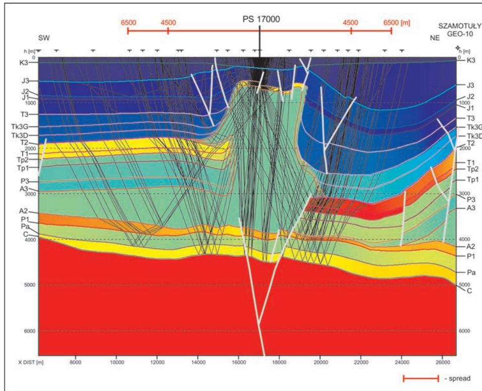
**Fig. 13.** Offset modelling: salt diapir, with two overhangs model (IV), PS 17000: Seismic ray trajectories
