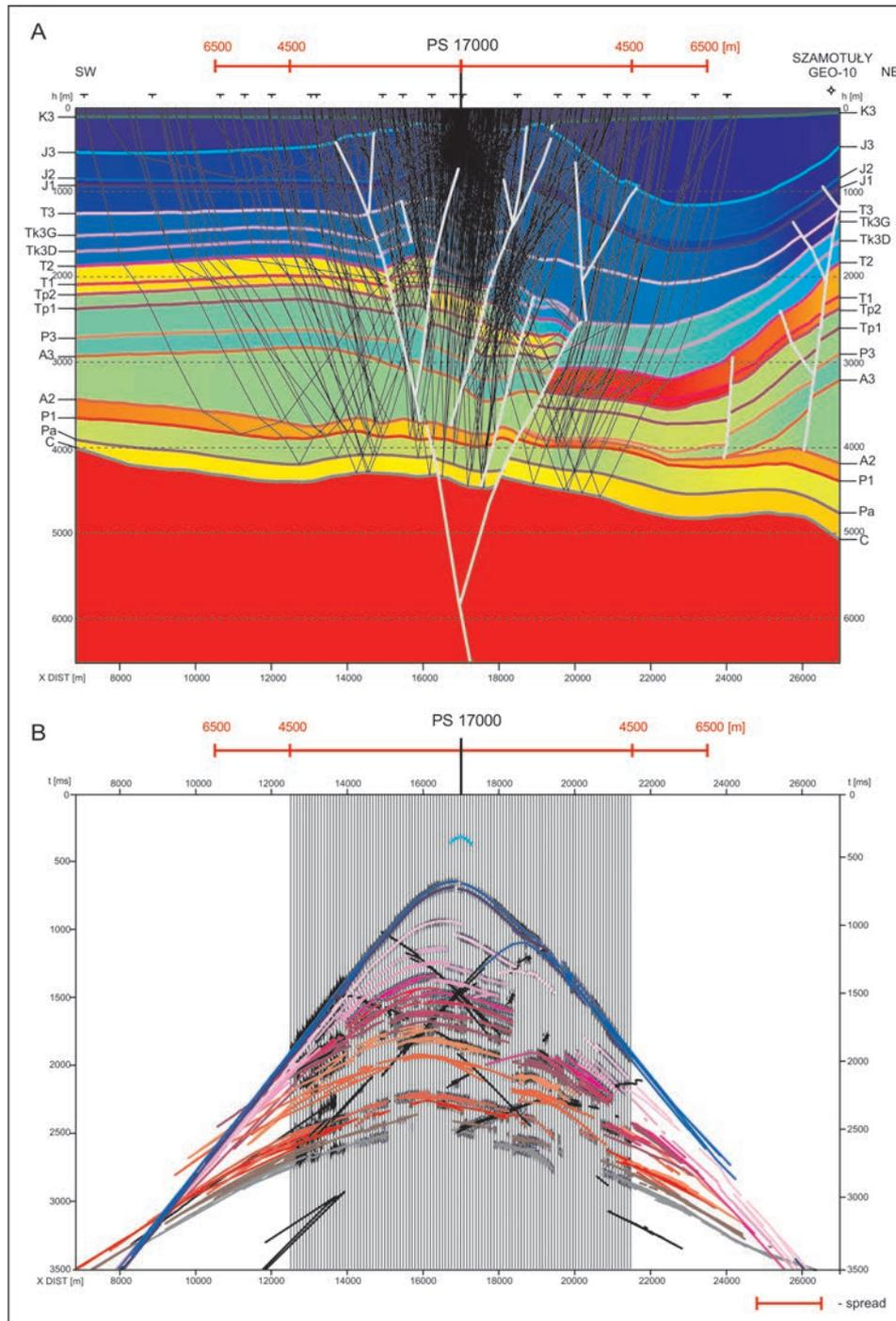
**Fig. 11.** Offset modelling: part of basic, seismic-geological model I (Szamotuly Zone), Ps 17000. **A** – Seismic ray trajectories; **B** – Seismic record. Colours marked as in Fig. 10C
