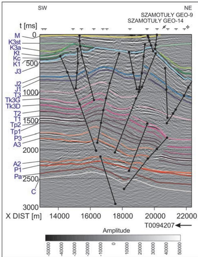
**Fig. 3.** Part of seismic transect, in which layer-block structure Szamotuły Zone (model I) was established. Seismic boundaries as in Fig. 2
