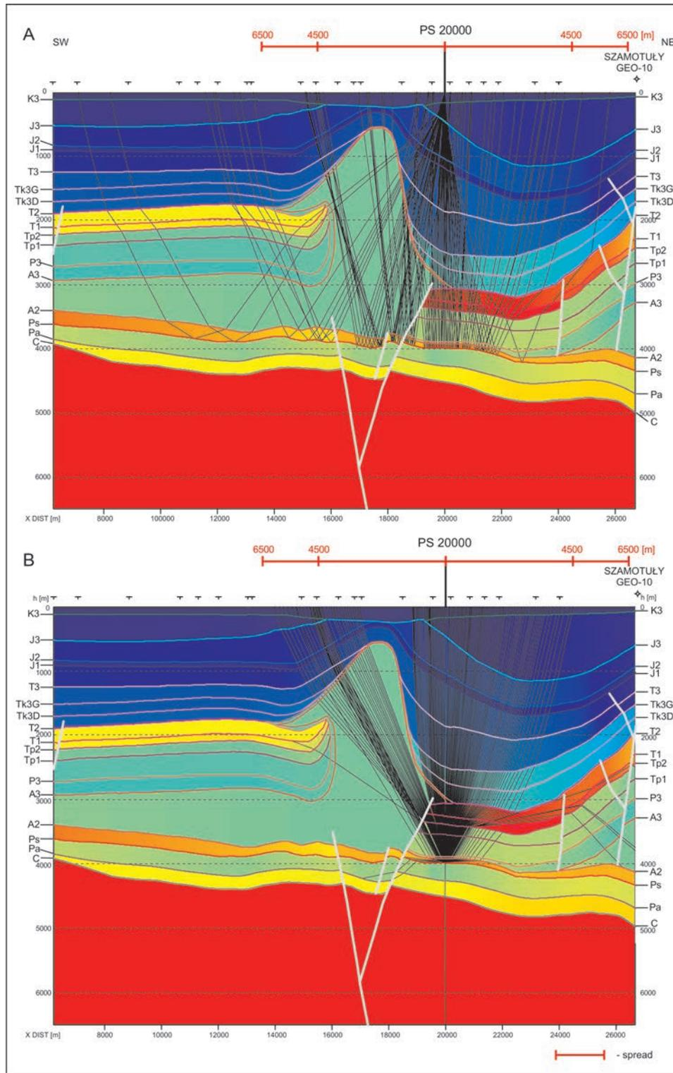
**Fig. 15.** Seismic ray trajectories, Szamotuły Salt Diapir model (V), PS 20000. **A** – shot record simulation; **B** – diffraction point (CDP gather simulation)
