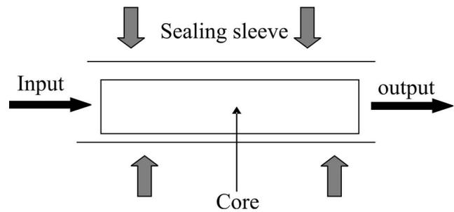
Fig. 5. Sketch of a measuring chamber
