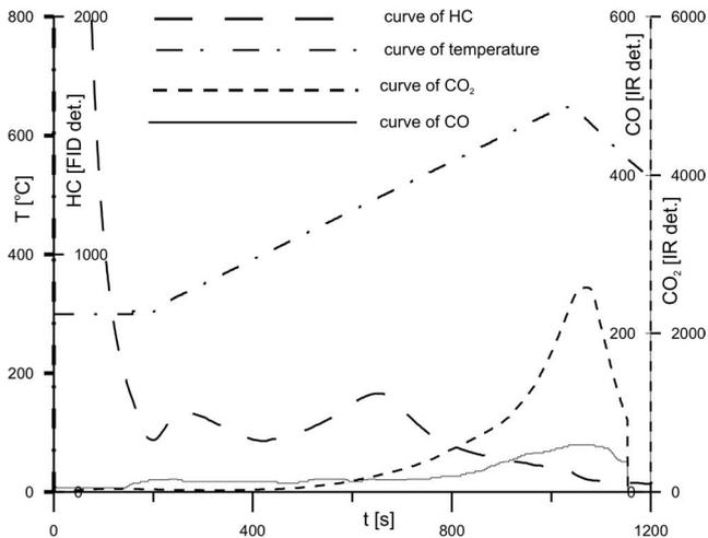
**Fig. 11.** Pyrolysis curves from Rock-Eval 6 illustrating presence of  $S_1$  peak and double  $S_2$  peak
