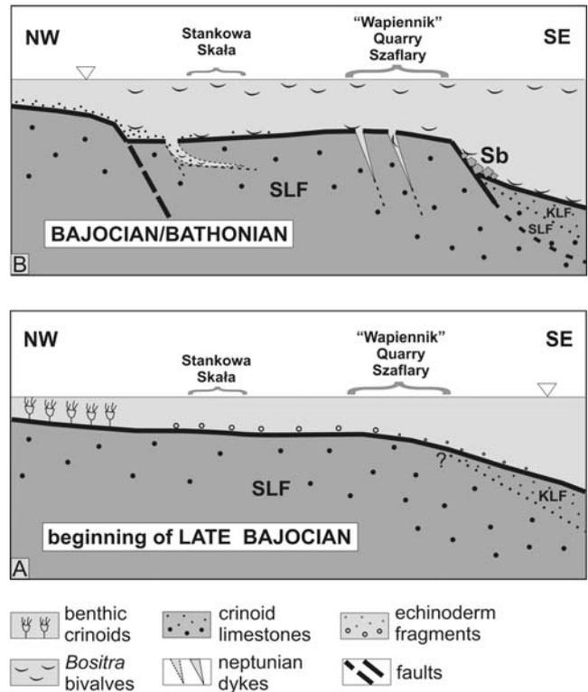
**Fig. 10.** Suggested geological evolution of the north-westernmost part of the Pieniny Klippen Basin with the southern part of the Czorsztyn Ridge. SLF – Smolegowa Limestone Formation; KLF – Krupianka Limestone Formation; Sb – scarp breccias (Wapiennik Breccia Member)
