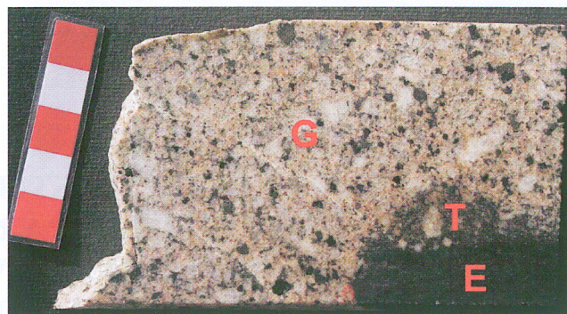
Fig. 2. Dark micaceous enclave in granodiorite from Będkowska Valley – borehole DB-5 depth 1370.0 m. E – enclave; T – transition zone; G – granodiorite
