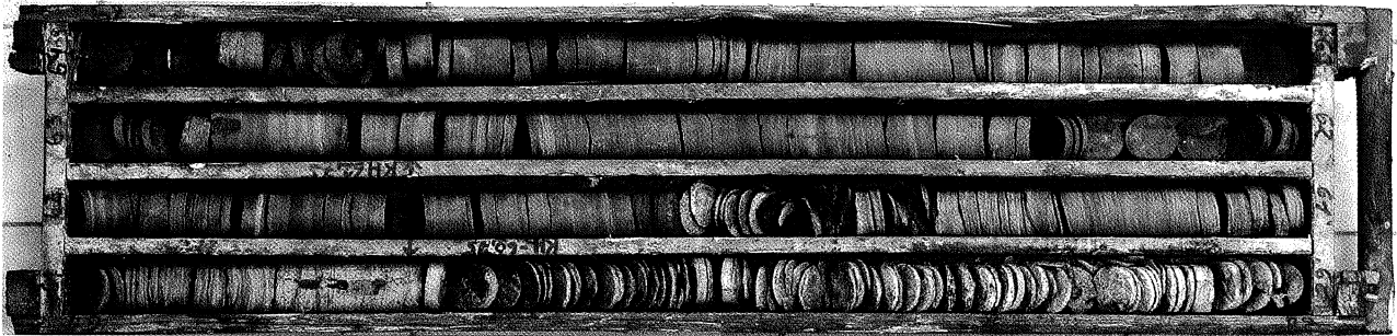
Fig. 1. Intervals of anomalous drillcore parting in boreholes ČSM 1152 and Staříč II - 750
