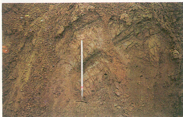
Fig. 16. Hinge zone of an upright open fold, cut by small-scale normal faults and joints. Central part of the Niedźwiedzia Góra pit
