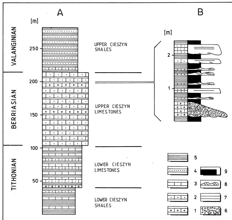
Fig. 2 A. Schematic lithostratigraphic profile of the Cieszyn Beds in Żywiec area. B. Fragment of profile with the layer of organodetrital limestones with ooids: 1 – limestone conglomerates; 2 – detrital limestones; 3 – pelitic limestones; 4 – calcareous sandstones; 5 – marly shales; sedimentary structures: 6 – massive; 7 – parallel lamination; 8 – ripplemark cross-lamination, 9 – structureless shale
