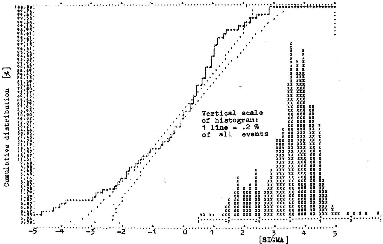
Fig. 8. Dry bulk density distribution for the sandstones from the whole Gorlice—Brzozów region
