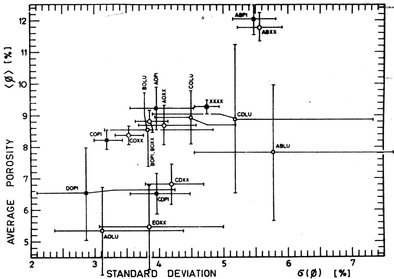
Fig. 4. Porosity distribution for sandstones KO from the Słopnice region
