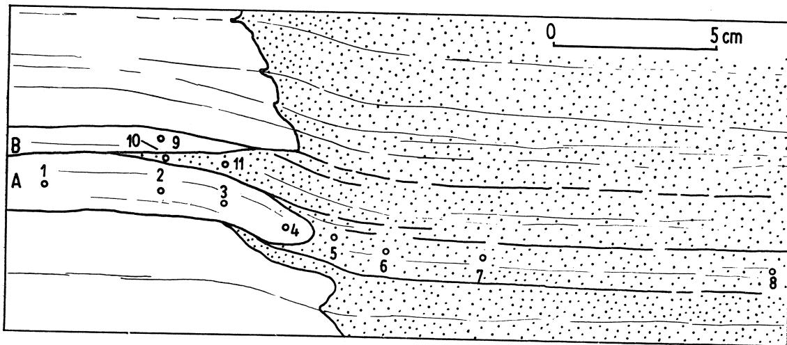
Fig. 2. Detail of contact between ore-bearing dolomite (dotted area) and Gogolin limestone shown in rectangular inset delineated in fig. 1. Numbers indicate location of analysed samples listed in Tabl. 3. A — layer of fine-grained limestone; B — layer of marly limestone, both A and B passing from unaltered relic to ore-bearing dolomite. Marly layer is slightly blurred in dolomite. Analyses of samples (Tabl. 3) indicate concentration of silica in dolomite close to contact with limestone
