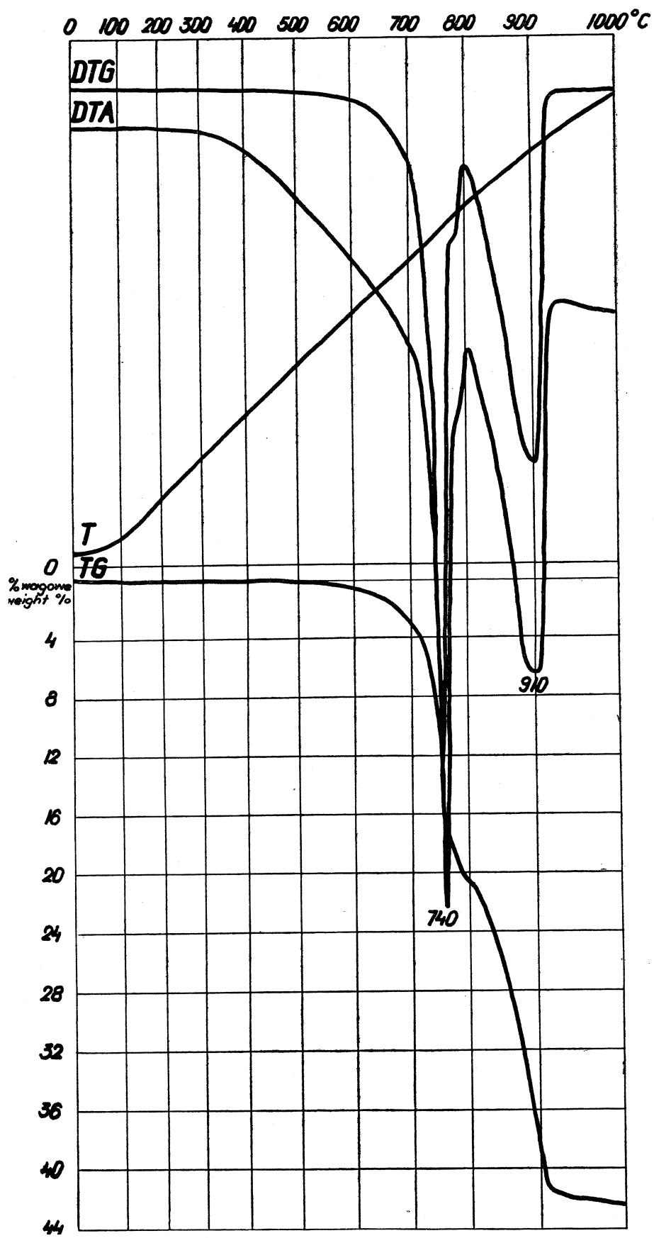
Fig. 4. Differential thermal and thermo-gravimetric analysis curves (DTA, DTG and TG) of primary Góraždje dolomite (0.5 g sample). Heating up to 1000°C in air atmosphere. Heating rate (T), 10°C/min. Derivatograph by F. Paulik, J. Paulik and L. Erdéy, produced by MOM, Budapest
