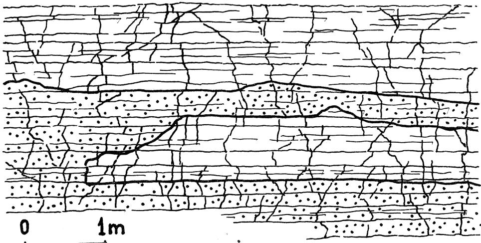
Fig. 3. Contact between ore-bearing dolomite (dotted area) and Górażdże limestone. Fragment of large limestone relic in ore-bearing dolomite. Compare Pl. L, fig. 2
